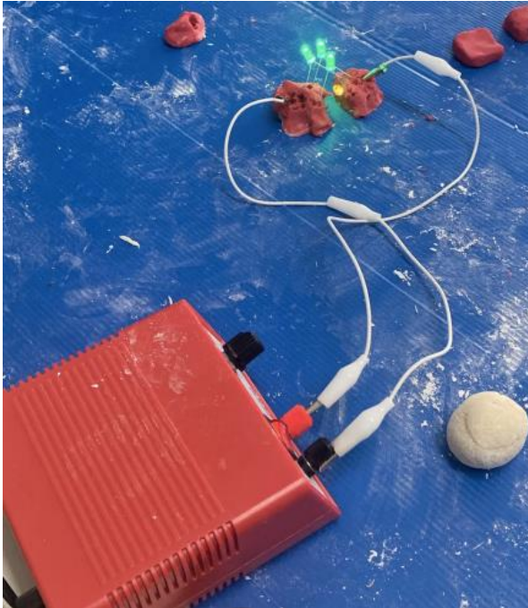
Figure 5. Parallel Circuit test using a low voltage adjustable power supply – (Andreas, 2020).
