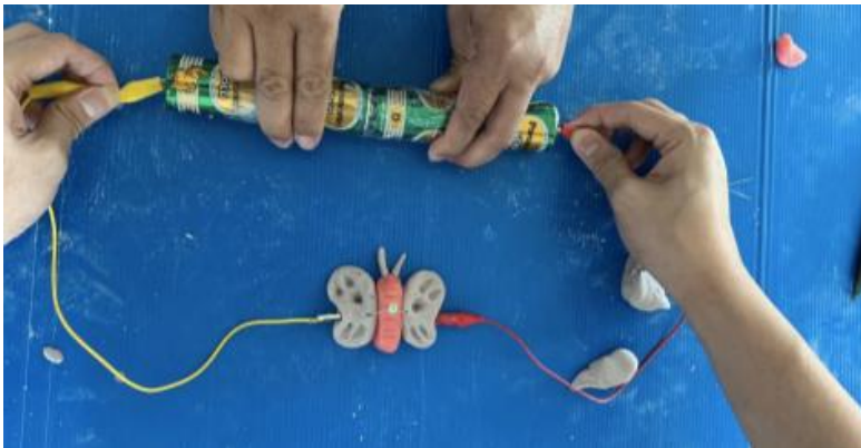
Figure 4. Butterfly Series Circuit – grey conductive dough, orange insulating dough (Andreas, 2020).
